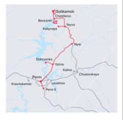
The project is aimed at accommodating the rising freight volumes of up to 23.0 mt in 2021 and up to 31.9 mt by 2025 by providing the Solikamsk–Perm Sortirovochnaya route for freight trains with a weight of 6 kt and a length of 71 standard cars.
