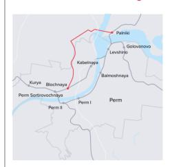
The investment project is aimed at accommodating the freight volumes from the Bereznikovsko-Solikamsky industrial hub by construction of a northern railway bypass of Perm with a railway river crossing over the Kama Reservoir.
